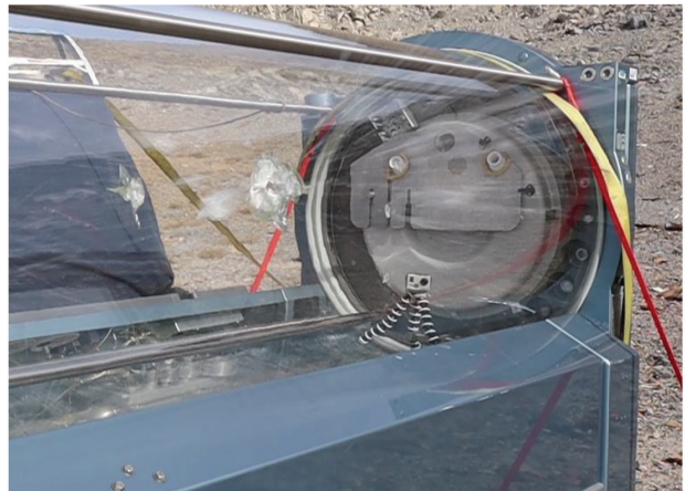
▲ FIGURE 5. Rapid depressurization after acrylic breach. A camera recorded the moment of impact at 120 frames per second. This frame rate was too slow to capture the bullet in motion or at impact, but the first three frames after impact are presented here.
