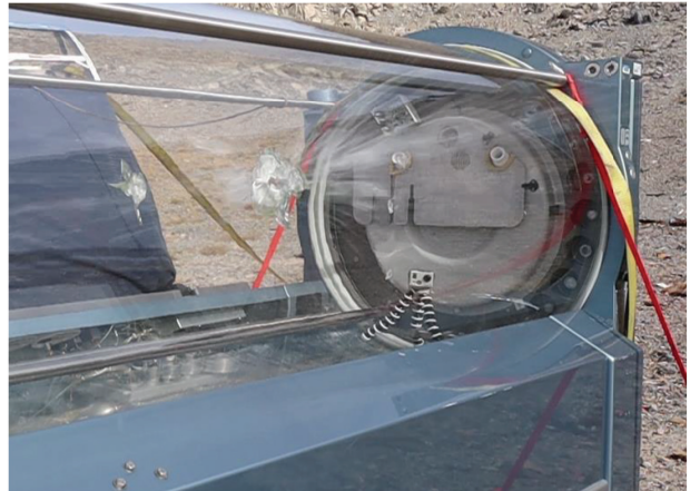
▲ FIGURE 3. Representative acrylic section showing damage from multiple impacts. This section underwent two rounds of testing with a .40 caliber handgun and 180 grain ammunition and required only two shots to break.
