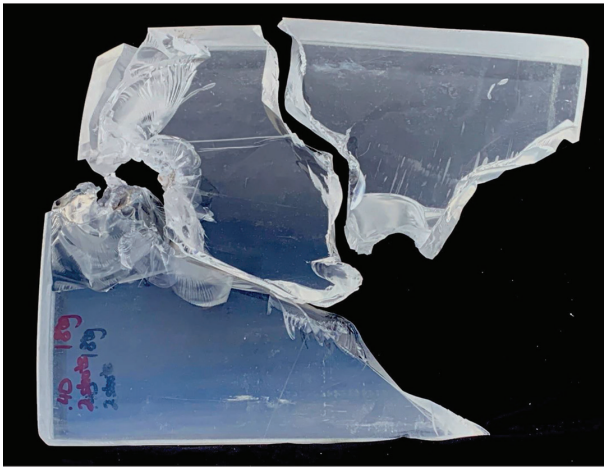
▲ FIGURE 3. Representative acrylic section showing damage from multiple impacts. This section underwent two rounds of testing with a .40 caliber handgun and 180 grain ammunition and required only two shots to break.
