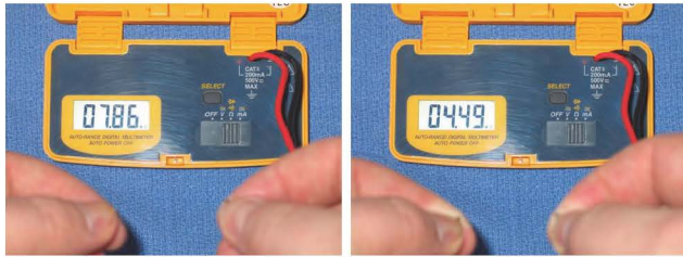
Probes Held Loosely ( 7.86 MΩ ) Probes Held Tightly ( 4.49 MΩ )
