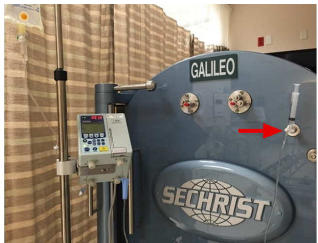
A Zyno Medical Z-800F pump infusing to a patient in a monoplace chamber. The pump's infusion set is attached to the proximal connector of a hyperbaric extension set that is sealed in the wall of the chamber (see arrow). Pumps must be able to generate 30 psi or more to deliver fluid into a pressurized chamber. Although it is depicted being used for a hyperbaric infusion, this model has not been FDA-cleared for such use. (Photo courtesy of Lindell Weaver, MD, Intermountain Healthcare, Salt Lake City, Utah)
