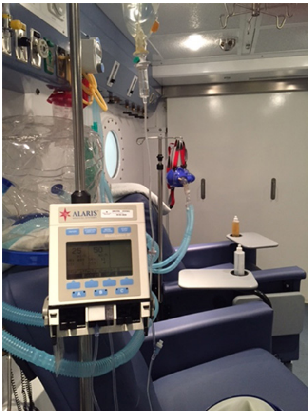
An Alaris MedSystem III pump set up for use on battery power in a multi-place chamber. Although it is depicted being used for a hyperbaric infusion, this model has not been FDA-cleared for such use. (Photo courtesy of Lindell Weaver, MD, Intermountain Healthcare, Salt Lake City, Utah)
